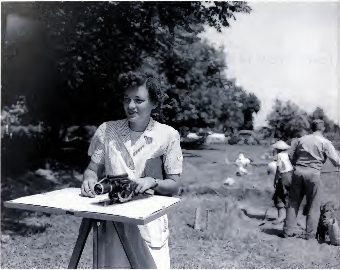
FIG. 14.1. Elaine Bluhm surveying with alidade and plane table at the Huber site outside Chicago, 1956.
